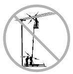
Keep away from machine if it contacts energized power lines or becomes electrically charged. Personnel on ground or in platform must not touch or operate machine until energized power lines are shut off.
