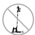
Do not operate the steer handle while the platform is occupied or raised.
