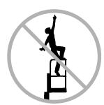
Do not exit platform while raised. If a power failure occurs, have ground personnel activate manual lowering valve.
