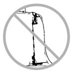
Do not cause a horizontal force or side load to the machine by raising or lowering a fixed or overhanging load.
